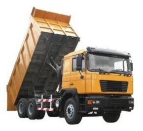
Application: tipper position detectionNeed: detection of the position of the tipper to avoid tip overHow: inclination sensor gives the exact position of the tipper
